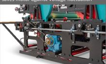
**Shaft Mechanism** drives each station with high grade steed made gear and shaft to give error-less printing registration.
