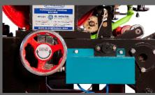
Do Not Dirty Belt System keeps the conveyor belt print-free during missed stock with sensor based auto-pneumatic system.
